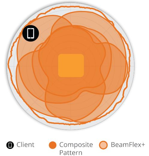
Figure 2. R750 2.4GHz AzimuthAntenna Patterns
